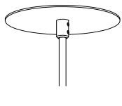
Mounting Option Power 1-5 Octagon Box (By Others) Installed in drywall, wood or concrete ceiling
